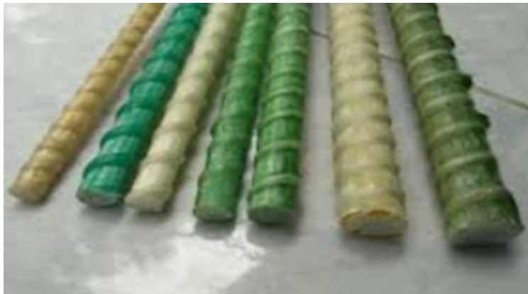
Figure 5: shows the use of fiberglass in reinforced beams.
